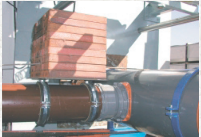
Shear loading test – 200 kg load
